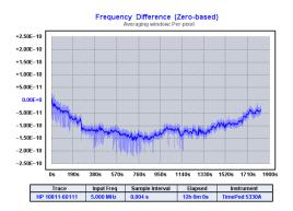
To sum up, selecting Measurement→Frequency difference (f), applying Subtract global linear frequency trend (drift line) (Ctrl-I), and enabling Trace→Phase/frequency traces begin at zero (z) can reveal details which are impossible to spot in the raw phase-difference trace. All of this being said, in order to get the same detailed view, we really only needed to enable Trace→Show linear phase/frequency residual (r) while viewing the frequency difference trace!
