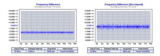
When used in the Measurement→Frequency difference (f) view, the effect of Trace→Phase/frequency traces begin at zero (z) is somewhat similar to applying Edit→Subtract global linear phase trend (frequency offset) (Ctrl-o) to each visible plot. It's not quite the same, though, because a trace's first data point is not necessarily anywhere near its trend line. Subtracting the trend will often do a better job at centering individual traces symmetrically about the Y axis, as seen below.
