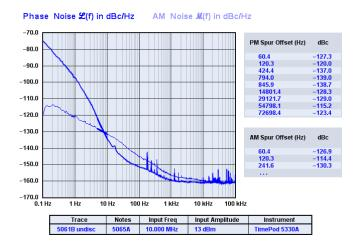
When enabled, this command renders a copy of the AM noise trace in the Measurement > Phase noise (P) view, using a lighter color or trace weight. Both PM and AM spur tables are displayed, space permitting.
