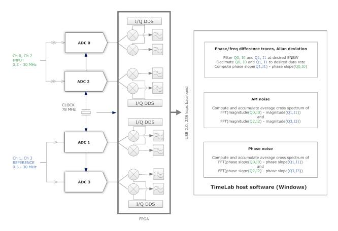
It can be helpful to understand some basic details about the TimePod 5330A's DSP topology, especially when measurements may be constrained by available memory and CPU resources. A key observation is that each of the three basic measurement types -- Frequency Stability, Phase Noise and Jitter, and AM Noise -- uses a completely separate data record and internal pipeline.
