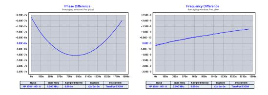
In fact, we could have achieved a similar effect without altering the phase record by viewing the phase-difference trace with Trace->Show linear phase/frequency residual (r), or by viewing the frequency-difference trace with Trace->Phase/frequency traces begin at zero (z). 10
