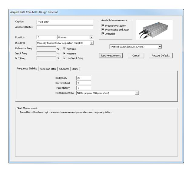
To get started, simply connect the 5330A's USB cable to your PC and launch TimeLab. Once TimeLab is running, select the Acquire→Miles Design TimePod menu option. The dialog box that pops up should contain a list of available TimePod device(s) in a dropdown box at upper right, just below the instrument photo.
