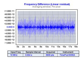
These two commands, Show linear phase/frequency residual (r) and Phase/frequency traces begin at zero (z), are among the most commonly-used options on the Trace menu. If you spend much time working with phase- and frequency-difference traces, their r and z keyboard shortcuts will quickly become familiar. z can increase visible
