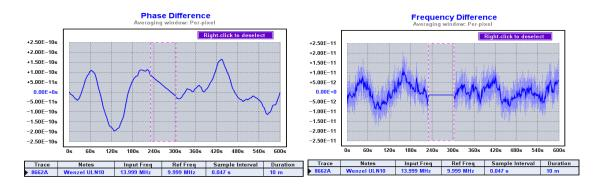
Above, the Flatten selected or zoomed phase data (Ctrl-f) command has replaced the selected region of the phase record with a straight line. The result appears as a flat spot in the Frequency Difference measurement view.
