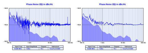
This command applies some light exponential smoothing to traces in the phase noise and AM noise measurement views. Detected spurs are always removed from smoothed traces. If enabled, smoothing is turned off automatically when the Trace→Suppress spurs in noise traces (Ctrl-s) command is used to toggle spur attenuation.
