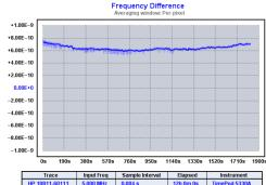
Essentially, Subtract global linear frequency trend (drift line) (Ctrl-I) removes the quadratic trend from the phase record, which has the effect of removing the *linear* trend from the frequency-difference plot. But there's still an arbitrary offset in the frequency-difference view that's forcing the Y-axis scale to +/- 1E-9, and the artifacts we'd like to examine are much smaller than this.
