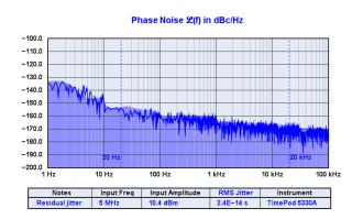
in phase noise plots are "integrated" as if they contained only random noise. Consequently, when viewing any of the RMS integrated noise values, you should use either Trace->Smooth noise traces (Ctrl-w) or Trace->Suppress spurs (Ctrl-s) to remove as much coherent energy as possible from the phase noise trace. Otherwise, time jitter and integrated-noise readings may be artificially exaggerated.
