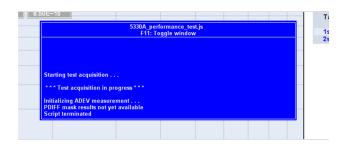
As the script console overlay tends to obscure the data being plotted, the F11 key provides a convenient way to hide or show the overlay for the currently-selected plot.
