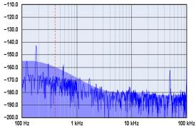
At left, the phase noise of a very high quality crystal oscillator has been measured over the course of several hours. Most of the visible spurs are well below the 5330A's specified limits, so it isn't clear which ones the instrument may be responsible for.
