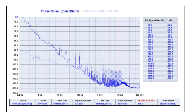
To measure the phase noise of a drift-prone source such as this HP 8640B cavity-tuned signal generator, uncheck the Frequency Stability option in the acquisition dialog. This will allow greater drift tolerance, since it won't be necessary for the signal to remain within a narrow measurement-bandwidth passband
