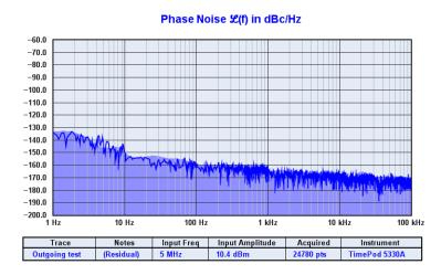
Phase noise and AM noise plots acquired with the TimePod 5330A and Symmetricom 512X analyzers can be displayed with a shaded area that provides an estimate of the instrument noise floor, if you enable Trace->Show estimated instrument noise (F2).
