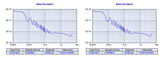
By default, screenspace points corresponding to the tau bins in Allan deviation and related statistical views are connected with a cubic spline. Spline interpolation results in a smooth, visually-appealing curve, but it can distort or exaggerate ringing artifacts and other abrupt transitions in the graph. When Trace Draw xDEV traces with spline interpolation (i) is toggled off, straight lines are used to connect the xDEV bins (above left).
