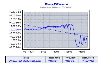
The trend line is not displayed in magnified views, or when Trace→Show linear phase/frequency residual (r) is enabled.
