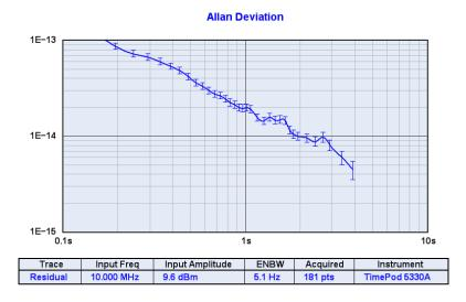
When enabled, this option draws "error bars" at each tau bin in Allan deviation and other statistical plots. These bars approximate the  $\pm$  one-sigma (68%) confidence interval at  $\pm$   $\sigma/sqrt(N/M)$ , where N is the number of phase-record samples that contribute to each bin and M is the bin's  $\tau_0$  multiple.
