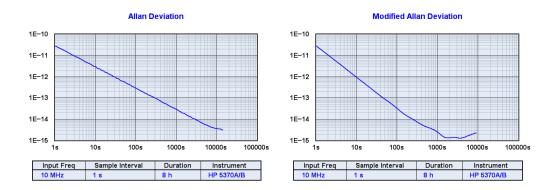
The ADEV plot shows a consistent  $\tau^{-1}$  slope to 10000 seconds, which could be indicative of either white PM or flicker PM noise. The MDEV plot renders the white PM noise at a slope of  $\tau^{-3/2}$ , transitioning to flicker PM near  $\tau$ =400s or so. Limited sample availability beyond  $\tau$ =2000s makes it difficult to draw further conclusions, but it's clear that MDEV reveals more about the counter's noise characteristics than ADEV.
