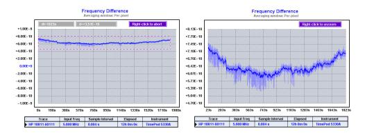
TimeLab is designed to take advantage of a PC mouse with three buttons and a scroll wheel. All of the graph types are "zoomable," and you can always return to the unmagnified view by right-clicking anywhere on the plot. Unlike the xDEV and noise measurement displays, though, the phase- and frequency-difference measurement views support additional navigation options. You can expand and contract the zoomed area with the mouse wheel, or surf through the data by dragging with the middle button.
