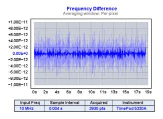
Of course, Edit > Subtract global linear phase trend (frequency offset) (Ctrl-o) has the drawback of altering the selected plot's phase data record and removing potentially useful information (namely the phase trendline). Fortunately, there's also a non-destructive global option that has the same visual effect, Trace > Show linear phase/frequency residual (r):
