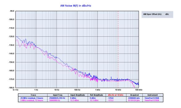
As expected, residual phase noise performance is improved when a strong 5 MHz signal is measured for 12 hours, compared to a weaker 25 MHz signal measured for 3 hours. The difference in AM noise isn't as pronounced in this case.
