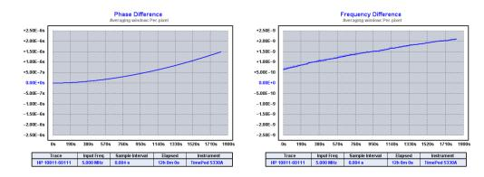
Not much detail is visible in either trace. Some sporadic frequency jumps are present, but they're not easily examined since their height is such a small fraction of the plot's overall magnitude. Subtract global linear phase trend (frequency offset) (Ctrl-o) command expands the phase-difference trace somewhat by removing its linear trend, but it only moves the frequency-difference trace down a bit:
