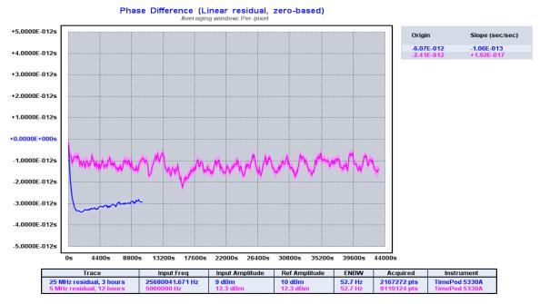
Despite visible HVAC cycling, overall phase stability is within +/- 1 ps over the entire 12-hour 5 MHz run.
