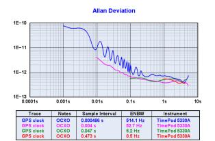
to appear on an ADEV plot, the antialiasing filter's response is easy to mistake for a real effect.
