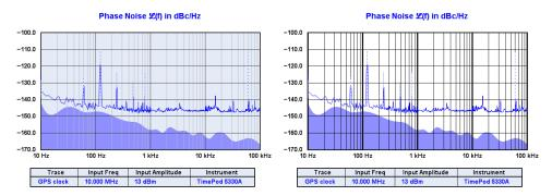
This command toggles between normal and high-contrast rendering. The latter option may be desirable when saving screenshots for publications or Web pages whose color fidelity may not be sufficient to reveal details in the plot such as minor graticule lines.
