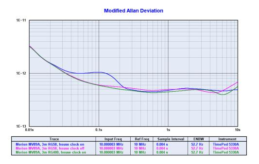
Crosstalk can also occur when a *third* signal, incidental to the measurement environment, causes beatnote effects that are asynchronous to both test inputs. This case is illustrated in the plot above, where a TimePod was used to measure a high-stability OCXO against another one of similar quality.
