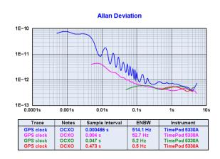
is simply the  $1/(2 * \tau_0)$  Hz Nyquist rate. This bandwidth is unachievable with a non-ideal antialiasing filter, so the 5330A driver internally acquires oversampled phase data that corresponds to an artificially short  $\tau_0$  interval relative to the selected ENBW. If allowed
